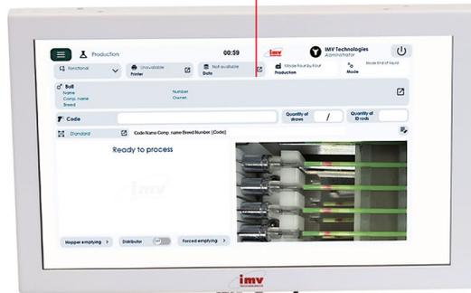
**Visual control from a distance** with on-board USB camera displaying live image on Supervision
